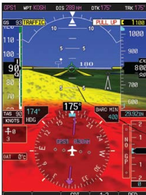
Figure 5-32 Synthetic Vision Imagery - PFD
